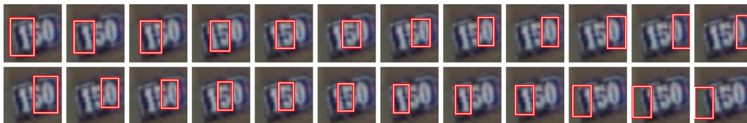
Figure 4.3: Example of an image processed by forward (top row) and backward (bottom row) models. Computation proceeds from left to right, i.e. the first step corresponds to leftmost image in each row. Image was taken from the test partition. Best viewed in color.
