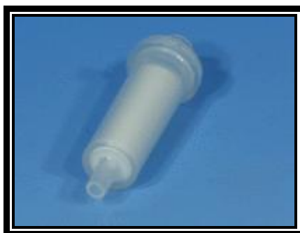
Figure 17. Chromafix C18 cartridges (Macherey Nagel) [66].
