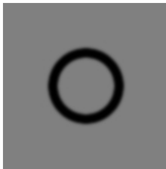
Figure 6.6.: Artificial image of a p-electrode used as reference for evaluating the correlation coefficient.
