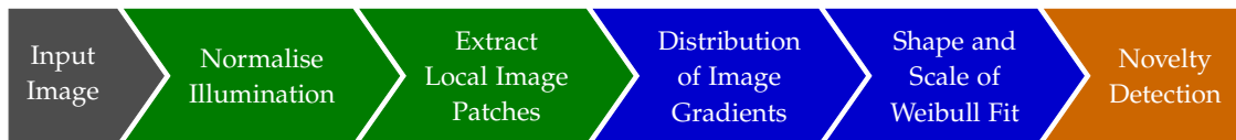
Figure 7.2.: Scheme of our novel system for detecting arbitrary defects in texture images.
